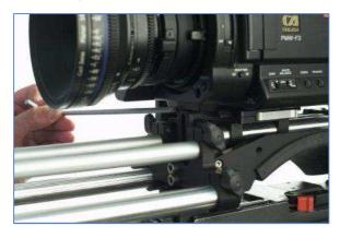
To set the correct support distance to the optics, unscrew the two hexagon screws (size 5.0 mm) and lift the 15/19 mm support interface until it touches the base of the F3 front. Then retighten the screws
