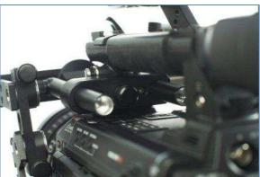
20) Mounting the articular arm to the finder tube and locking the arm and the handle tube
