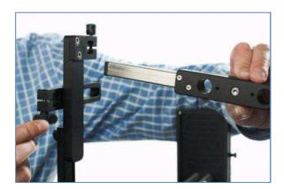
5) Unscrew the three lower screws using two different hexagon keys (sizes 3.0 mm and 2.0 mm). The telescopic side part can then be completely removed
