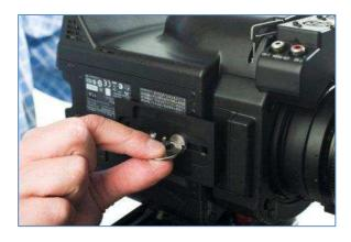
8) Unscrew the two black button screws at the side of the quick release and move the camera slide. On the Sony F3 to about a finger's width in the direction of the front end of the two tubes
