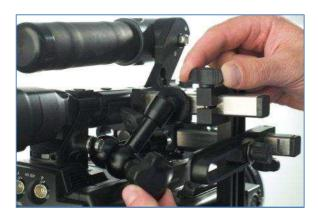
Push the finder rods as far back as possible and lock using the black button screws which are located on the rear side between the two finder rods
