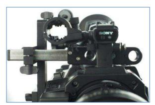
17) Remove the handle tube of the top handle
